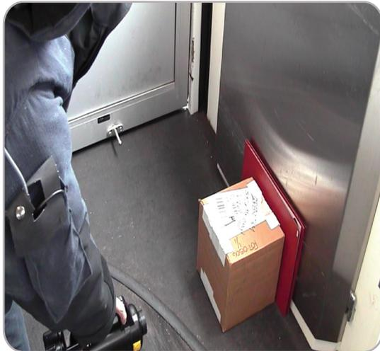
**Scanna ScanX Scout is the lightest, most portable and rugged CR style x-ray system with flexible image plates for getting into confined spaces or taping onto or around larger surface areas. The imaging plates are available in a range of sizes from 8" x 10" to 14" x 17" as well as custom longer lengths. The optional Quad Plate allows you mount up to 4 Image Plates to check larger targets such as suitcases.**
